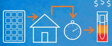
Further maximise the full potential of the iStore by syncing it with a solar power system. The easy-to-use, built-in smart timer will offset any excess power to the iStore, saving you even more.
