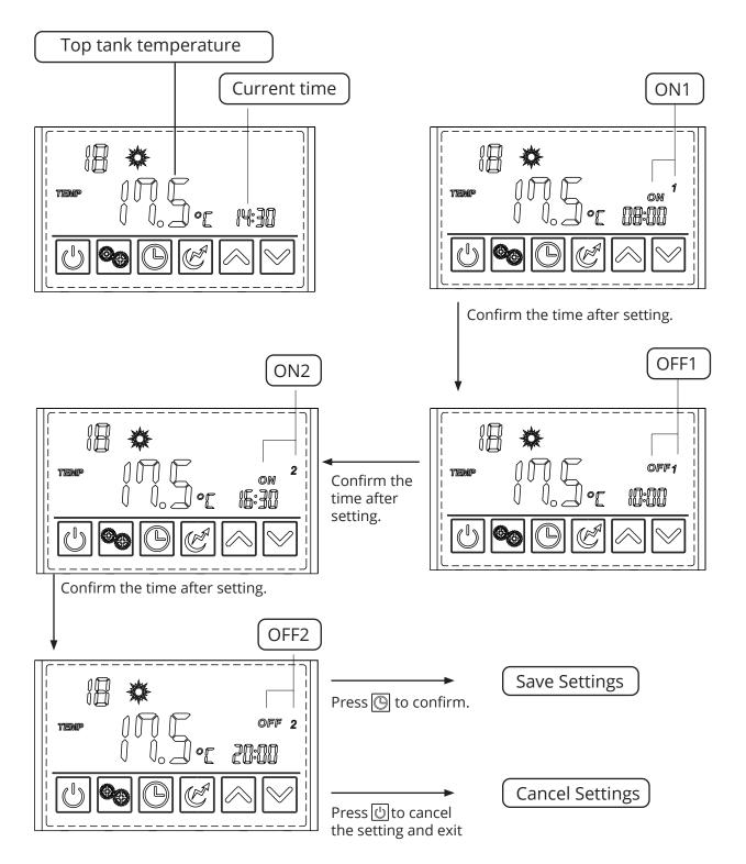
NOTE: Do not set the second timer to 00:00 ON and 00:00 OFF as the unit will commence heating at midnight every second night. To leave the second time off simply allow the timer setting to time-out after setting the first timer end time.
