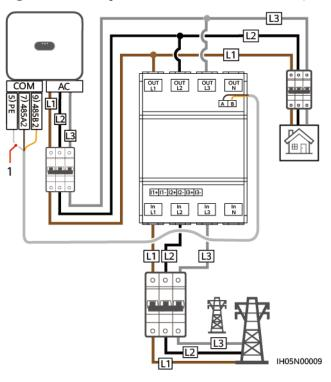
Figure 5-23 Three-phase, three-wire direct connection (Smart Dongle networking)
