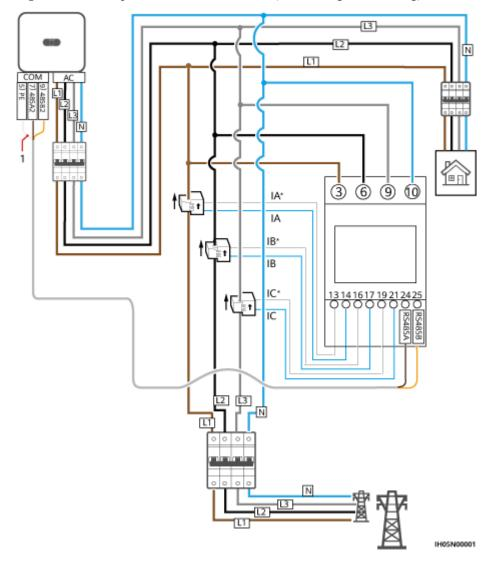
Figure 5-22 Three-phase, four-wire connection (Smart Dongle networking)
