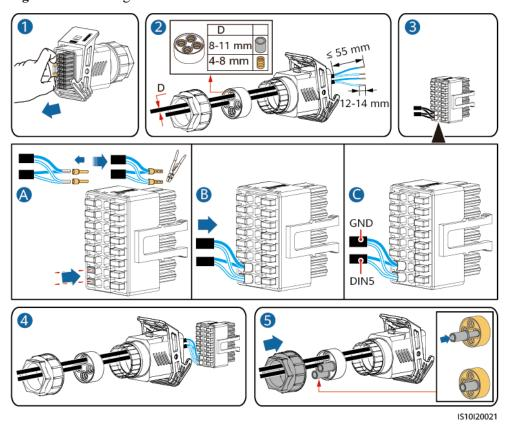
**Step 2** Connect the signal cable connectors to the COM ports.
