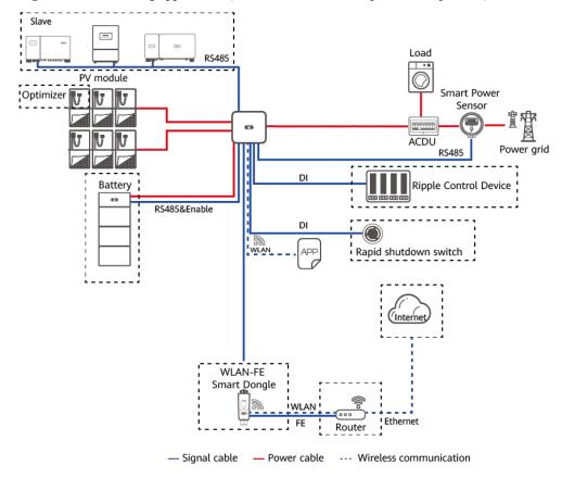
Figure 2-1 Networking application (dashed boxes indicate optional components)
