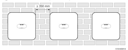
Figure 4-4 Staggered installation (recommended)
