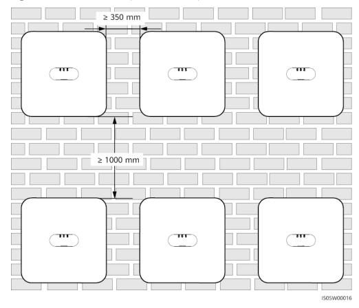
Figure 4-5 Stacked installation (not recommended)
