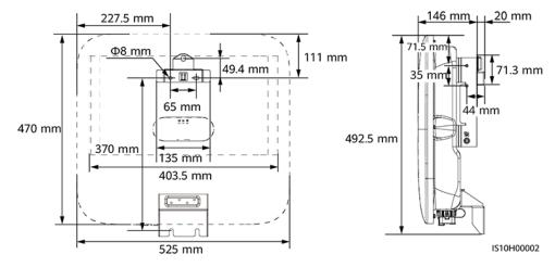
Two M6 screw holes are reserved on both left and right sides of the enclosure for installing an awning.
