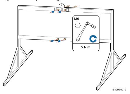
Step 4 (Optional) Install the locking screw for the DC switch.
