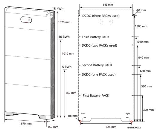
Figure 5-2 Floor-mounted installation dimensions
