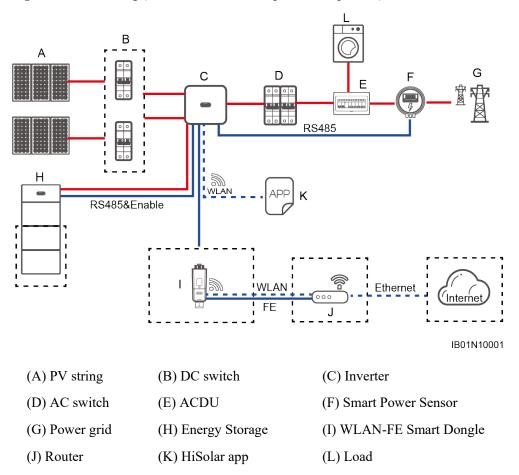
Figure 2-2 Networking (dashed boxes indicate optional components)
