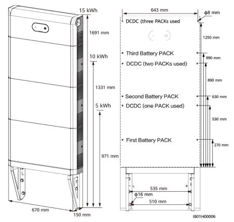
Figure 5-7 Wall-mounted installation dimensions
