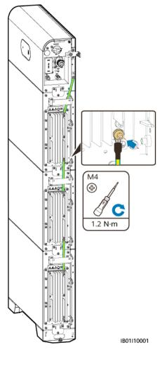
Figure 6-2 Connecting the internal PE cable
