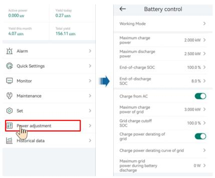
Figure 4-5 Battery control parameter setting
