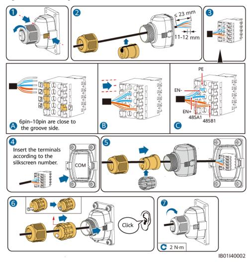
Figure 6-15 Connecting inverter terminals
