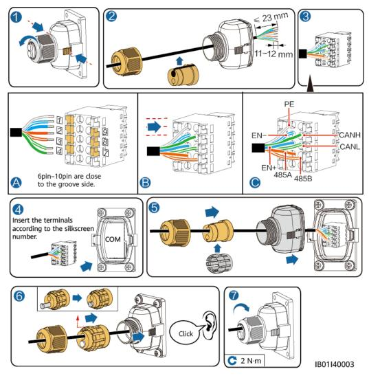
Figure 6-18 Cascading communication terminal
