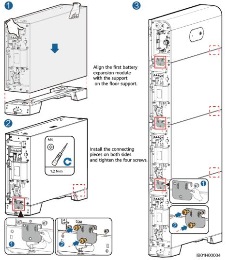
Install the remaining battery expansion modules and power control module from bottom to top.
