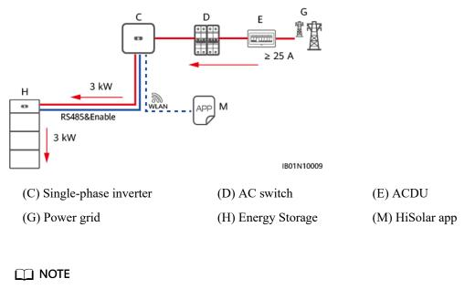
Figure 8-2 Networking diagram for single-phase power supply scenario
