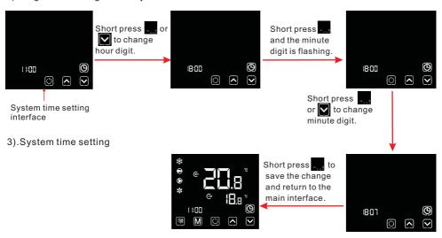
Notes: After the permanent awakening of clock key, if it is not cancelled by user, the main interface will display the clock key permanently. Under the clock setting interface, if short press , the change will not be saved and return to the main interface; if there is no operation for 20s, the system will automatically memorize user's setting, and return to the main interface.
