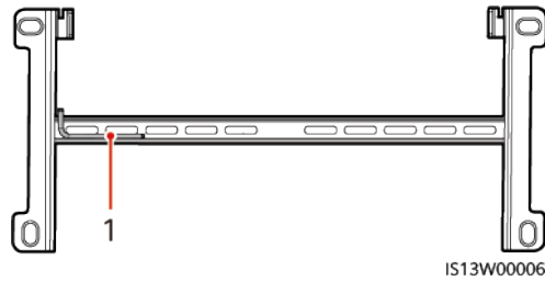
Figure 4-9 Position for binding the security Torx wrench
