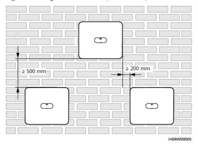
Figure 4-4 Triangle installation mode (recommended)
