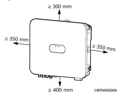
• When installing multiple inverters, install them in horizontal mode if sufficient space is available and install them in triangle mode if no sufficient space is available. Stacked installation is not recommended.
