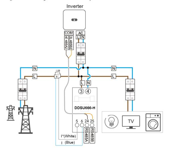
Figure 5-28 Connecting cables to the DDSU666-H power meter
