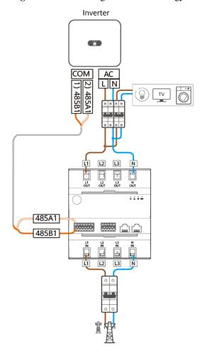
Figure 5-20 Connecting cables to the Energy Management Assistant
