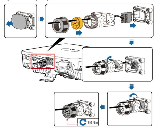
Figure 5-33 Securing the signal cable connector
