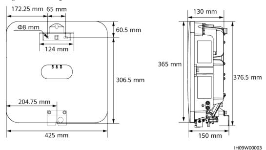
Reserve enough clearances around the inverter to ensure sufficient space for installation and heat dissipation.
