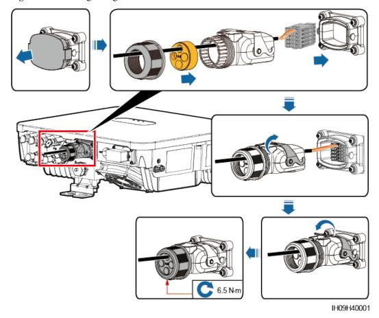
Figure 5-19 Securing the signal cable connector
