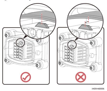
Figure 5-17 Installing the connector block
